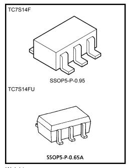
Weight SSOP5-P-0.95: 0.016 g (typ.) SSOP5-P-0.65A: 0.006 g (typ.)
